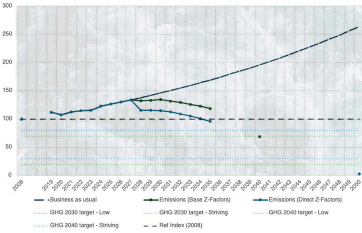
Figure 3. Projected evolution of total GHG emissions from international shipping (indexed to 2008 = 100) – assuming 3% annual growth.
